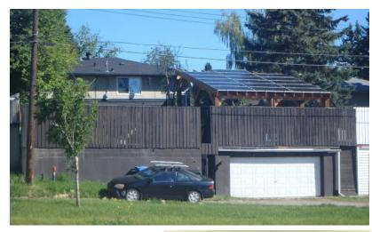
constructed) below. The PV system on top of the garage not only powers the cars and home, exports to the grid, but also serves as a cover for the deck below. The bi-facial panels are chosen for the deck to still have a bit of sun exposure while maximizing the production of panels.
